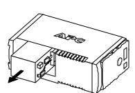
b. Pull the battery about half way out, as shown
